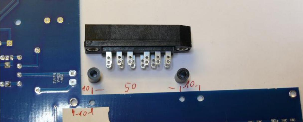
Then connect the female connector to the main board using attenuator pads (VHF-choke + 100 Ohms resistor in parallel ) as already depicted. Use heat shrink tube to assure that everything is well insulated. Connect all outward going screws to ground.
