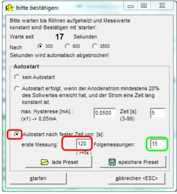
After the first measurement a second measurement cycle is automatically started from the RoeTest.
