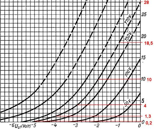
The characteristic curve's pairs of values are entered in the evaluation window at the item "add curve" (red marked fields), with increasing x-values ("gesendete Spannung [sent voltage]") from the left to the right. Empty fields will represent the value pair 0/-99. There is one specific peculiarity to observe: It is not possible to represent an anode current of 0mA. You have to enter a very small value (e.g. 0,01mA) instead of 0mA.
