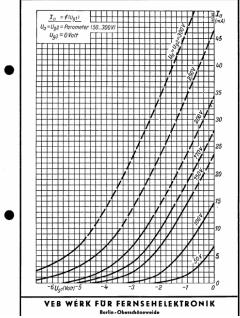
Excerpt from the data sheet of an EF80 given as a PDF file:
