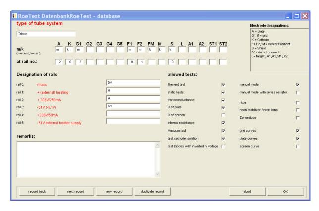
In this file the tube type is entered, for example diode, triode, pentode...
