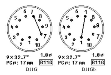
The numbering differs from the data sheets (1-11) due to the connection of pins. The pin assignment in the database for gnom tubes is only valid in conjunction with the above tube base pictures.
