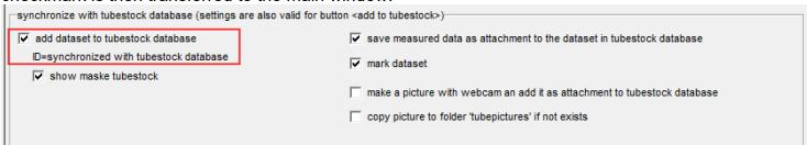
The tube is added to the inventory database in batch processing. There is the option of saving the measurement data there (if the checkbox "save measurement data as attachment to the dataset in the tubestock database" is checked.
