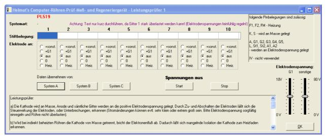
Each socket pin can alternatively be assigned to the heater supply, 0V, positive voltage G1 or to positive voltage "sonst."; it can also be left unconnected. There are two slides to control the level of the voltages. Using the buttons <System A> (B,C) allows to import the socket connection scheme of the currently loaded tube data.
