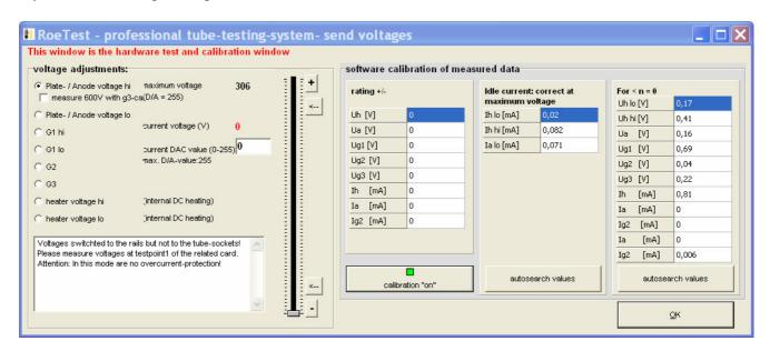
Used for testing and adjustment of the hardware (voltage sources and measuring instruments). The voltages must be measured at the boards, test point 1, using a multimeter (for adjustment see the building instructions). Those voltages are not switched to the tube holders.
