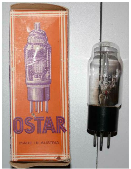
At the beginning of the 1930ies the company Ostar (Gustav Ganz, Vienna) produced so called high voltage tubes. The voltage of the filament was designed so that the filament could be directly supplied from the mains voltage. The heating transformer or a series connection and series resistors were unnecessary for that tubes.
