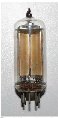
The tube has no heater but only anode and cathode. Operating voltage is 50 V. The maximum current is 10µA.
