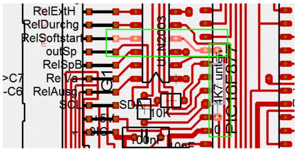
A 12 V relay is mounted near the mains connection and the coil is connected to the positive relay supply and the VG connector. The relay will bypass the NTC some seconds after switching on.
