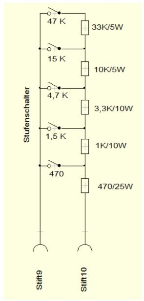
The resistors need not be very precise as they are only used for current limiting.
