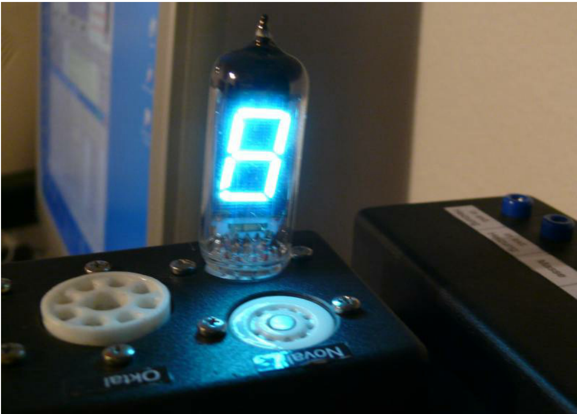
All segments of a VFD glow equally bright. With the slider the brightness of the display can be controlled.
