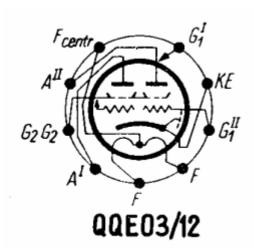
As he socket diagram shows, the screen grids of both sections are connected to pin 7.
