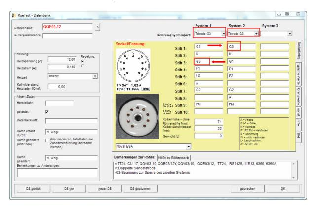
The tube type "Tetrode-G3" is selected for both systems. As you can see, as each section is measured, the control grid of the other section is connected to the G3 negative-voltage source.
