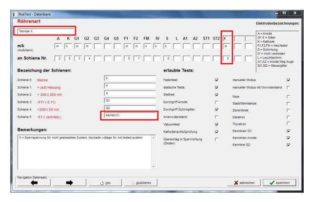
Here an electrode (X) is defined. This electrode is assigned to rail 5 (the second negative-voltage source in RoeTest).
