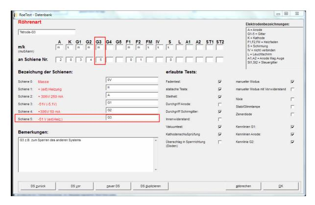
Here an electrode (G3) is defined, even though the tube type is a tetrode with no suppressor grid. This electrode is assigned to rail 5 (the second negative-voltage source in RoeTest).
