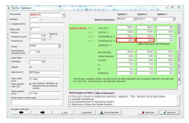
In the tube data, the X voltage is set to the high negative value of -50V.
