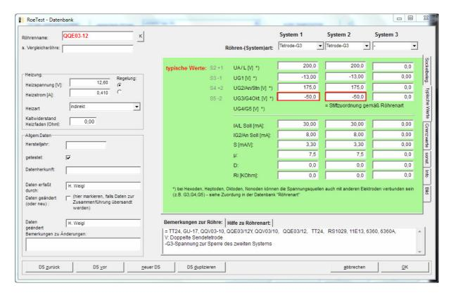
In the tube data, the G3 voltage is set to the high negative value of -50V.
