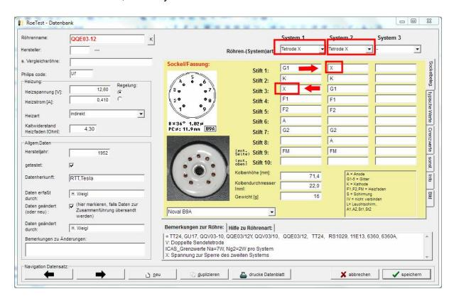
The tube type "Tetrode X" is selected for both systems. As you can see, as each section is measured, the control grid of the other section is connected to the X negative-voltage source.
