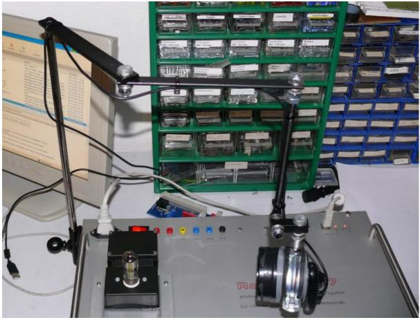
My monopod is simply made of some flat iron and round iron tubes, threaded rods and a bunch of nuts, bolts and washers. The monopod is attached using a pipe clamp.
